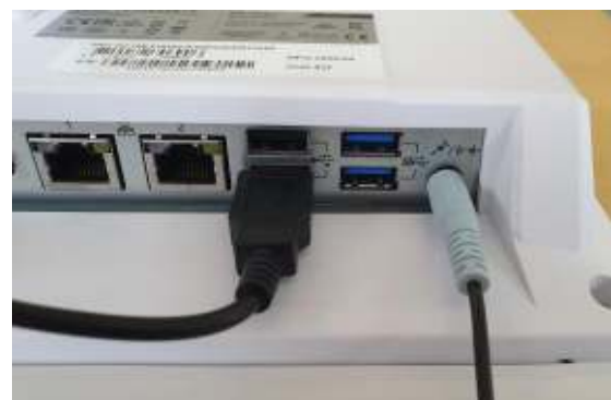
Connection to USB & Combo Audio Socket ...
