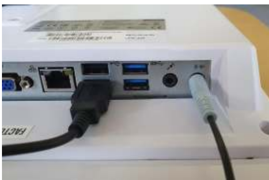
Connection to USB & Audio Out Socket ...
